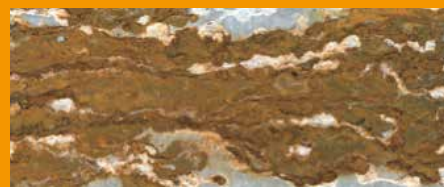
Conventional galvanisation after 6 weeks in a salt spray test
